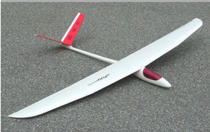
**Phillip 600 Sport** -- This is a nice 2-meter slope model for light to medium winds. Would also make a good warmliner electric model if you want to chop of the nose. Fiberglass fuse, obechi over foam wing, built up V-tail. Two piece wing, removable tail so the model breaks down nicely for travel. Includes 4 servos for ailerons and V-tail. Flown a few times, still in excellent condition. \$195
