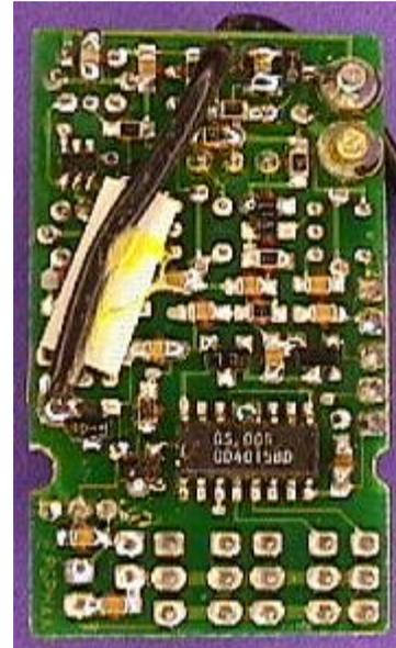
Rear view of 535 circuit board. 16 pin chip between the two notches in the board is the one you want to find.
